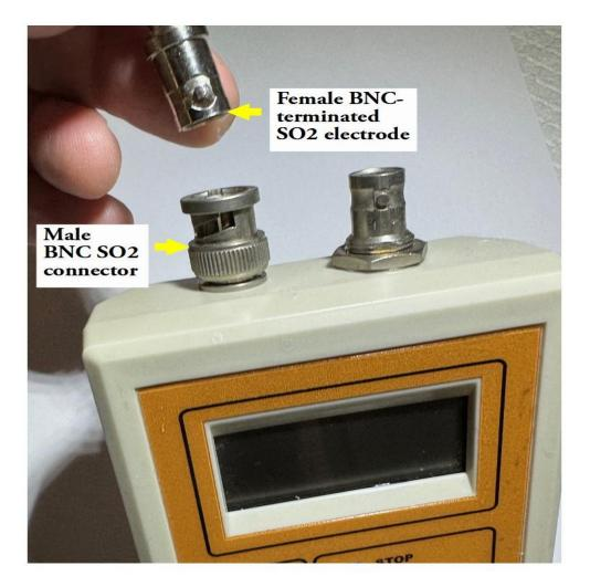
Our most current SO<sub>2</sub> connection type. This connection type eliminates any possible issues with regards to connectivity, while also being different enough from our pH connection port so that there is no way to attach electrodes to the incorrect port.
