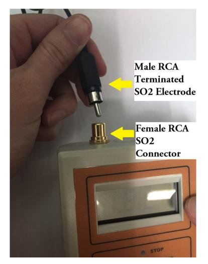
Our second SO<sub>2</sub> connection type. [Note: Occasionally, we have had customers who had trouble getting a good connection using their RCA terminated SO<sub>2</sub> electrode. This problem can be remedied by taking a pair of pliers and ever so gently squeezing the Male RCA Electrode outer ring. This allows for a better connection and eliminates any connection issue.
